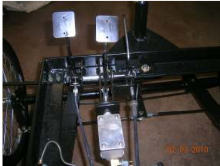
Clutch and gas cables connected to the pedals.
