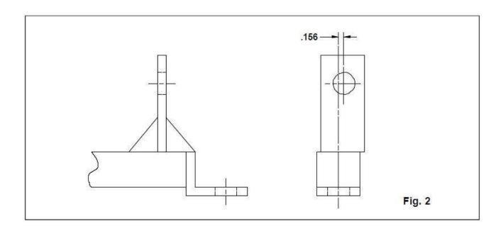
I added a feature, shown in Figure 2, to Pete's idea. By making the top mounting hole off 5/32" to the rear of car, we get 3 degrees positive caster.
