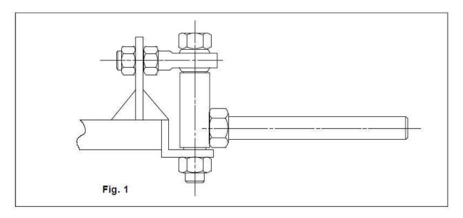
Figure 1, above, depicts Pete Burger's neat way of making the camber adjustable on a typical "homebuilt" front axle. The top of the kingpin is supported by a 5/8" ball type rod end. By adjusting the nuts holding it, the camber can be fine-tuned as desired.
