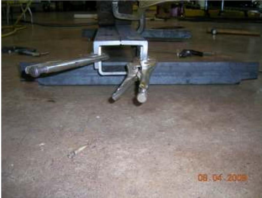
I marked the angle iron for one set of springs front and rear, and carried it over to my mill and drilled the 3/8" holes. Once this was done I installed the spring to that one side. I then put the other set of springs beside this set and marked the axle mounting holes with layout dye, and scribed a straight line through the holes.
