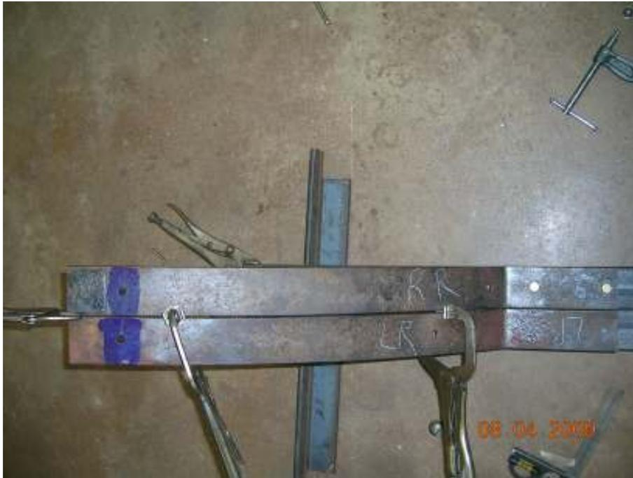
After I had the springs properly aligned I marked the other side rail, and drilled it also on the mill. I installed the last pair of springs on the rail to make sure they were properly aligned with the other pair, and then removed the springs so I could weld the frame.
