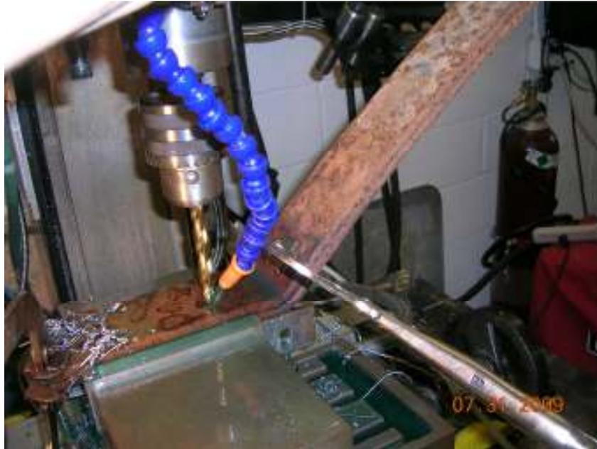
It really wasn't that hard to drill. I used 400 RPM and plenty of coolant.
