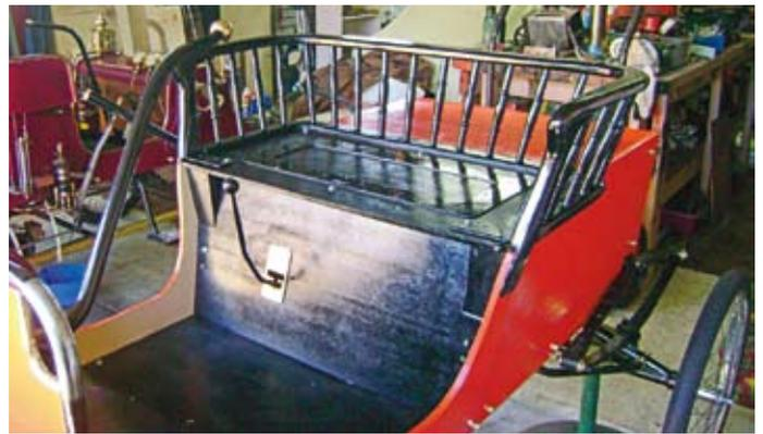
the wooden spindles which I turned up by eye on my metal lathe. The spindles were made from old jarrah tomato stakes and the lathe has benefited from this exercise as all the worn slides are now filled with wood dust! The hand rails are angled out more than the original to give more bum space. The original looked pretty narrow to me.
