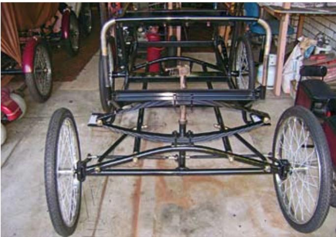
the springs to sag over a period of time without further heat treatment and if that happens I'll rip them out and repeat the cold hammering process. Chassis is of a welded construction and is made up from 50mm x 25mm box section steel. The body panels are made from 12mm thick marine ply sheeting.
