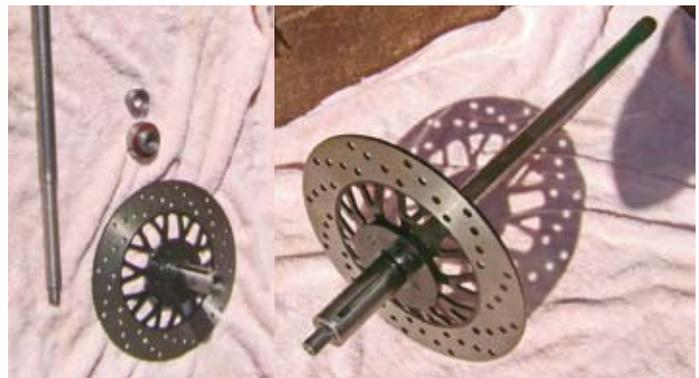
motor bike and the master cylinder is from the Mazda referred to earlier. The master cylinder is of the dual system type so I just paralleled up the outputs into a single line since I only have rear brakes and much to my surprise it works beautifully.
