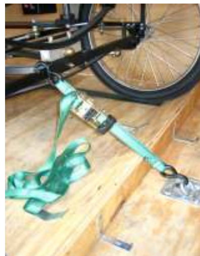
Front tires resting on front angle stop. Strap holding car against front stop
