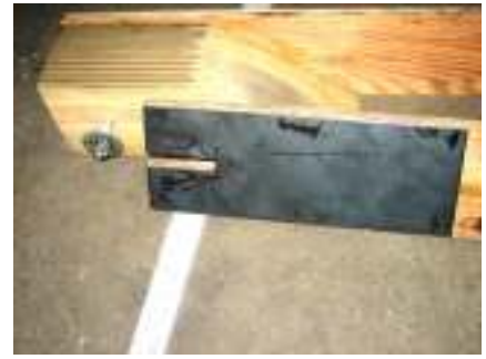
Slotted steel plate on left wheel lock (slips on the stud under the washer)
