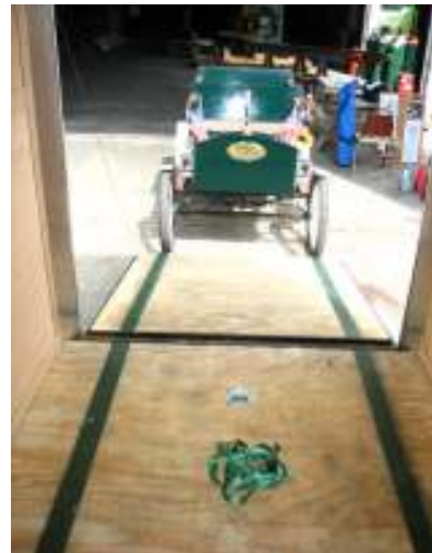
Loading & Unloading drive guide lines on ramp & floor, “D” ring in floor at rear door of trailer for rear ratchet strap.
