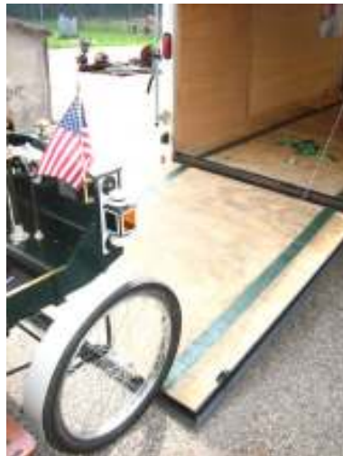
Loading & Unloading drive guide lines on ramp & floor, “D” ring in floor at rear door of trailer for rear ratchet strap.
