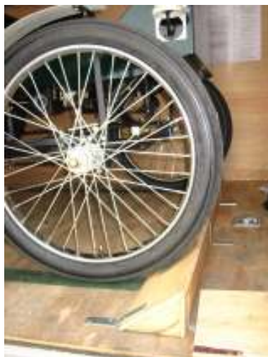
Front tires resting on front angle stop. Strap holding car against front stop
